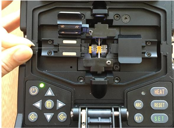
2.6.1 Open shielding cover and left and right fiber clips.
