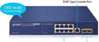
8 x Gigabit 802.3bt PoE++ Port 2 x 100/1000BASE-X SFP Slot
