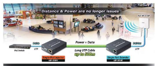
Extend IP Ethernet transmission and inject power beyond the 100 meters
