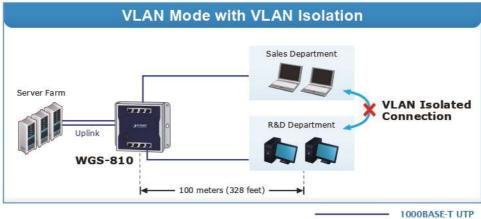
In the **Extend operation mode**, the WGS-810 operate on a per-port basis at 10Mbps duplex operation but over a distance of up to 250 meters overcoming the 100m limit on Ethernet UTP cable. It also supports VLAN isolation to isolate ports so as to prevent broadcast storm and defend DHCP spoofing in the extend operation mode.
