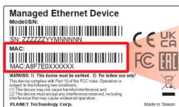
Figure 4-2: Industrial Managed Switch MAC ID Label
