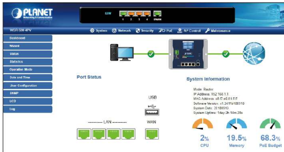
Figure 5-3: Web Main Screen of Industrial Router
