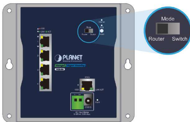
Figure 5-5: WGR-500 DIP switch button
