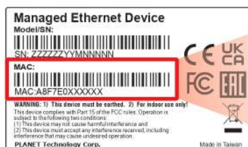
Figure 5-3: Industrial Managed Switch MAC ID Label
